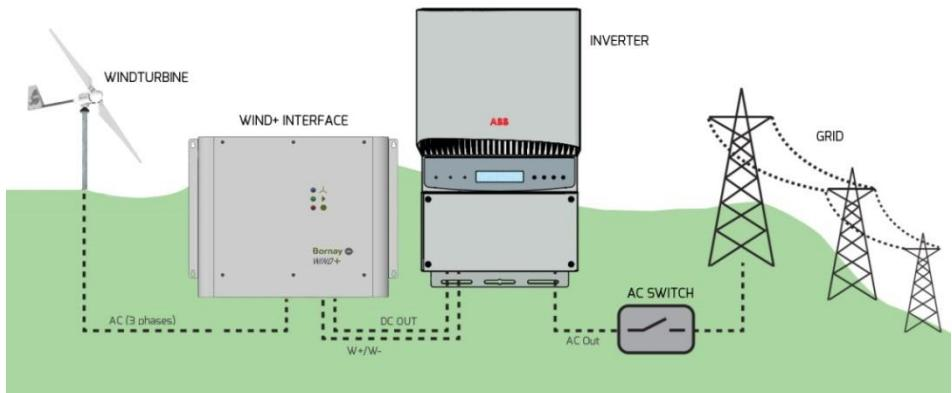
Data connection between the interface and the ABB inverter
